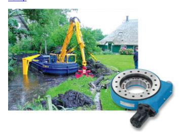
This work boat which is used in Dutch canals is fitted with a WD-L series Slew Drive to move the boom of the excavator.
