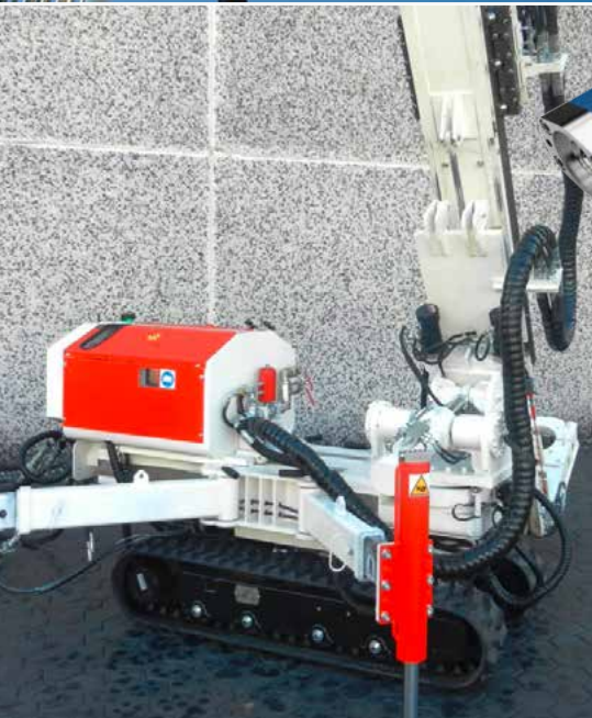
Drilling booms whose horizontal drilling linkage is taken into position using a slew drive from the WD-L range (two drives)
